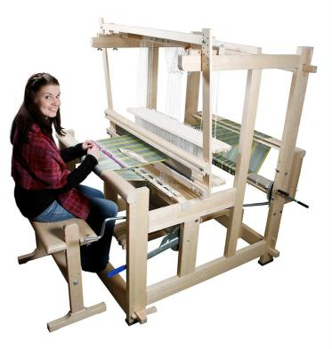
The large side opening allows for easy access to warp and tie-up.
