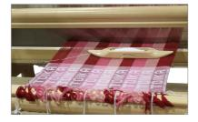
The ES control unit, contained in a sleek and beautifully designed outer case, is directed by the computer and software to select the appropriate shafts and open the shed automatically. The shed is a true countermarch - the shafts that are programmed to rise do rise and those that are programmed to sink do sink. Sheds are also even throughout as the ES unit automatically compensates for the shafts that are farthest from the weaver.
